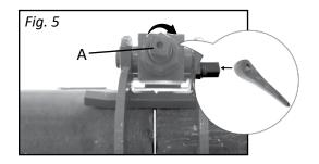
**4.** Close clamp onto pipes by tightening down on the ratchet bolt. (*A, Fig. 5*)
