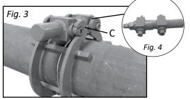
**3.** Place clamp in middle of pipes to be welded. (Fig. 3) Insert ratchet into holding ears. (C, Fig. 4)
