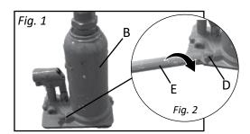
**1.** Release all pressure from hydraulic cylinder (*B*, *Fig. 1*) by turning release valve. (*D*, *Fig. 2*)
