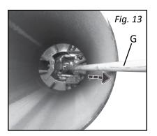
6. Turn crank handle clockwise (G) until clamp is fully expanded inside pipes. (Fig. 10) Note: Clockwise = tighten, counterclockwise = loosen
