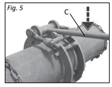
**1.** Lift hand lever (C) to release the hand lock placement (A) free
