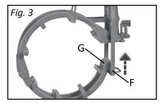
**2.** Lift tension rod (F) from clamp end. (G, Fig. 3)
