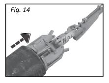
**10**. Pull clamp through secondary pipe joint. (Fig. 14)
