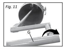
**7**. Turn crank handle clockwise *(G)* until clamp is fully expanded inside pipes. *(Fig. 11)*
