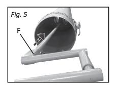
**1**. Insert appropriate length of reach rod (F) through pipe joint. (Fig. 5)
