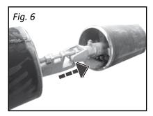
**2**. Place clamp into the pipe joints to be welded. (Fig. 6)
