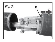
**3**. Pull on clamp until stop (B) catches. (Fig. 7)
