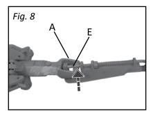
**4**. Clip hook (E) onto Input shaft eye. (A, Fig. 8)
