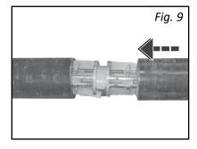
**5**. Move secondary pipe onto clamp. (Fig. 9)
