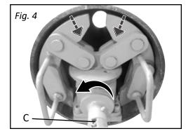
. Turn crank handle (C) counterclockwise to fully close and remove Pipe Expander. (Fig. 4)
