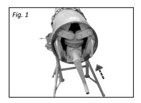
. Insert Pipe Expander into pipe. (Fig. 1)
