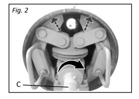
. Turn crank handle (C) clockwise until pipe rests are fully depressed. (Fig. 2)
