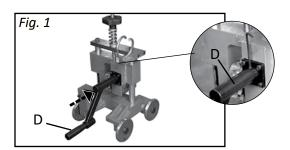
**1.** Attach Crank Handle (E) to the Chain Beveling Machine by mounting to the post and tightening with the 3 mm hex key
