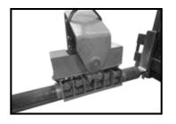
1. Place bending shoe over pipe to be bent
