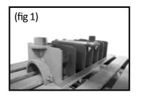
1. Cut off (2) support rods before installation and operation of bending shoe (fig 1)
