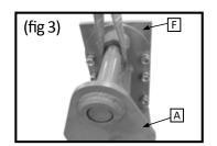
3. Bolt mounting bracket (A) to mounting plate (F) (figure 3)
