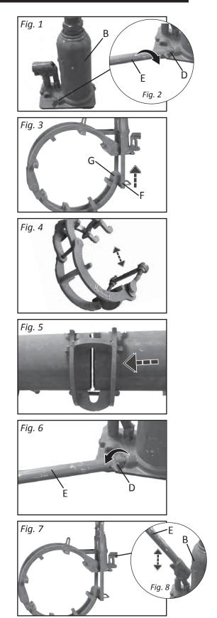
**1.** Release all pressure from hydraulic cylinder (*B*, *Fig.* 1) by turning release valve. (*D*, *Fig.* 2) Note: Use hydraulic handle (E).
