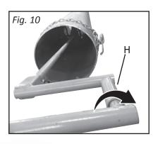
**6**. Turn crank handle (H) clockwise until clamp is fully expanded inside pipes. (Fig. 10)
