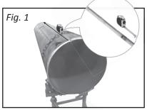
**1**. To find appropriate length of reach rod (G), measure pipe joint to be welded. (Fig. 1)
