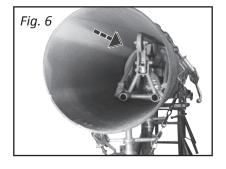
**2**. Place clamp into pipe joint. (Fig. 6)
