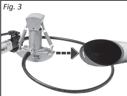
1. Insert the Hydraulic Dent Remover so that the head and base of the Hydraulic Dent Remover are in line with the Short Diameter of the pipe. (Fig. 3)
