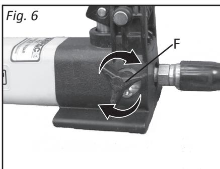
4. Relieve the pressure by turning the hydraulic release valve (F) on the Hydraulic Dent Remover and lower the head of the reformer. (Fig. 6)
