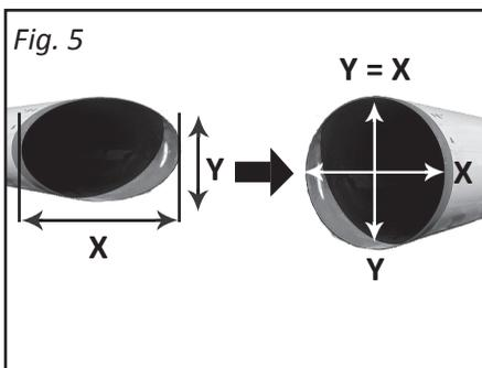
3. Increase the pressure on the Hydraulic Dent Remover until the short diameter of the pipe (Y, Fig. 5) measures the original long diameter of the pipe. (X, Fig. 5)
