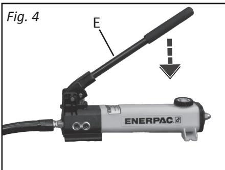
2. Use the hydraulic pump (E) to increase the hydraulic pressure. (Fig. 4)
